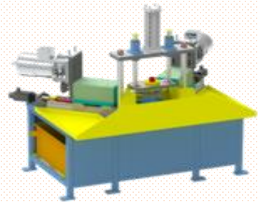
Pipe facing SPM
